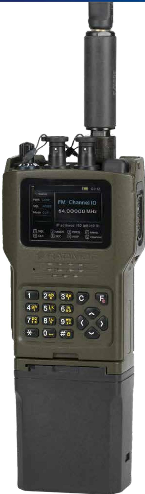
The COMP@N H08 is a SDR handheld radio, developed using a common hardware platform for all COMP@N family radios. This COMP@N radio has implemented a frequency hopping waveform (W2FH), which allows simultaneous transmission of voice, data, SA (Situation Awareness) and GPS reports.
